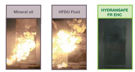
ISO 20823 Hot Manifold Ignition Test at 600  $^\circ\text{C}$  : In this test, an oil leak on a hot spot of 600  $^\circ\text{C}$  is simulated.
